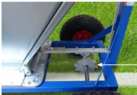
TAMIS VIBRANT ENTRAÎNÉ PAR ROUE DENTÉE FIXÉE SUR L'AXE DES ROUES ARRIÈRE
